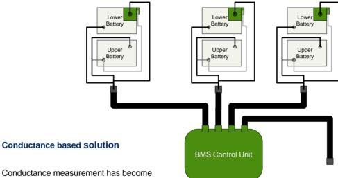
Conductance measurement has become established in the automotive and standby power industry as the only reliable method for quantifying the health of a lead acid battery.
